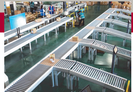
Large multi-station sortation handles a variety of parcel sizes.
